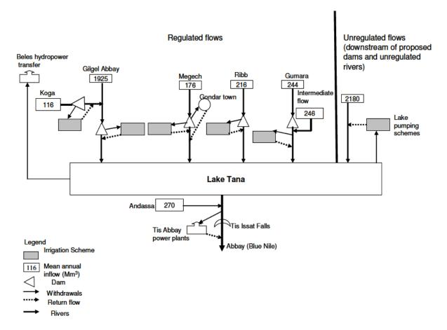
Figure 5: Scheme of existing and planned water development schemes (source: Alemayehu et al. 2009: 9)
