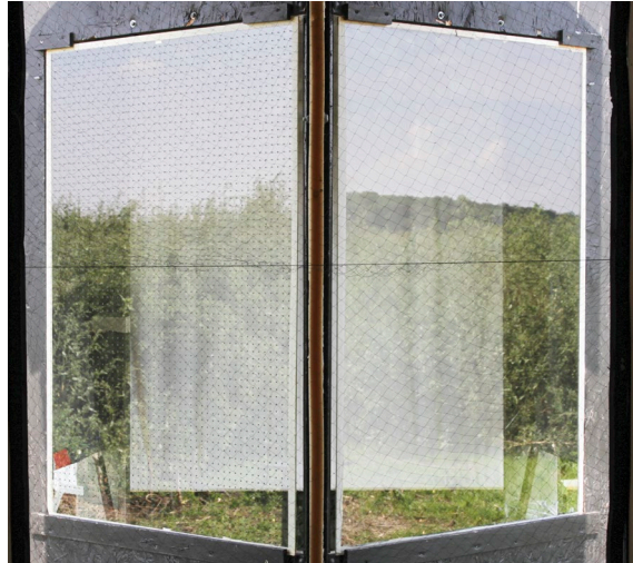
Despite the small spacing between dots, this dot grid is ineffective: a dense grid of black dots with 3 mm diameter was not recognised by birds even on surface 1 (left: test pane, right: reference pane).
